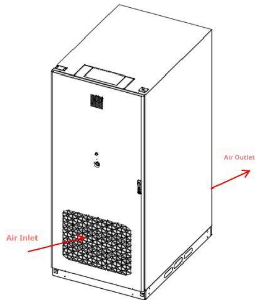
Figure 5- 2 Illustration of Equipment Air Inlet and Outlet
